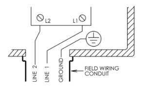
**ATTENTION:** ROUTE WIRING DIRECTLY FROM FIELD CONDUIT TO TERMINAL BLOCK AS SHOWN. DO NOT BUNDLE EXCESS WIRING INSIDE DRIVE ENCLOSURE.
