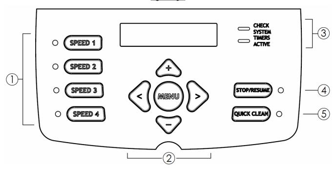
1. **Preset Speeds:** Buttons labeled SPEED 1 thru SPEED 4 can be used to run the pump at a predetermined speed for a certain length of time. Preset Speed settings can be quickly updated using the + and - arrow buttons to change the speed and then pressing the > button to save the new speed setting. When a speed is selected, the LED beside the button will illuminate to indicate operation.
