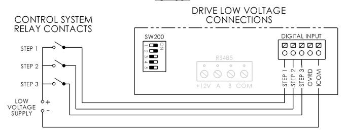
Connection wire must be rated for a minimum of 300V. Inputs are rated to accept a low voltage supply of 18-30VAC (24VAC+/-20%) or 9-30VDC (12/24VDC +/-20%). The "+12V" and "COM" terminals may be used as a low voltage supply, however, these terminals also supply power to the user interface, so care must be taken when connecting to these terminals to ensure proper operation of the user interface. SW200 DIP switch #1 and #2 must be "ON".
