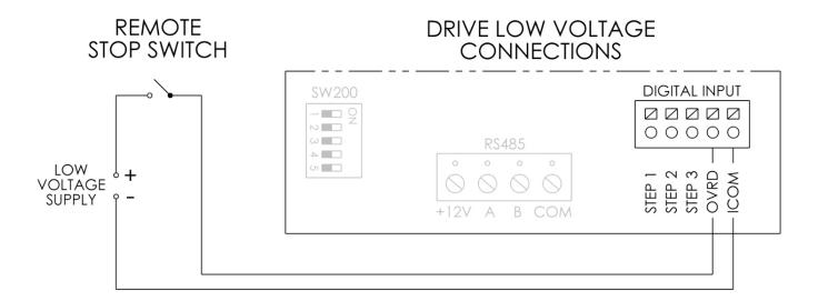
Connection wire must be rated for a minimum of 300V. Switch must be latching type; pump is stopped when circuit is closed. Inputs are rated to accept a low voltage supply of 18-30VAC (24VAC +/-20%) or 9-30VDC (12/24VDC +/-20%). The "+12V" and "COM" terminals may be used as a low voltage supply. For SP3200VSP, these terminals also supply to the user interface, so care must be taken when connecting to these terminals to ensure proper operation of user interface.
