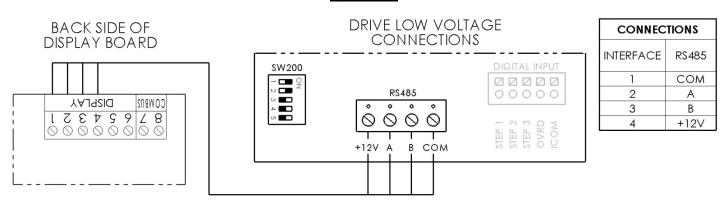
Connection wire must be rated for a minimum of 300V, and may be up to 500 feet in length. Use removable 4-position terminal block connectors for wiring connection to interface and motor drive PCB's taking care to note the wire colors and corresponding numbers next to the connectors. **Terminal block must** be installed with screws facing up to ensure proper connection. SW200 DIP switch #1 and #2 must be "ON".
